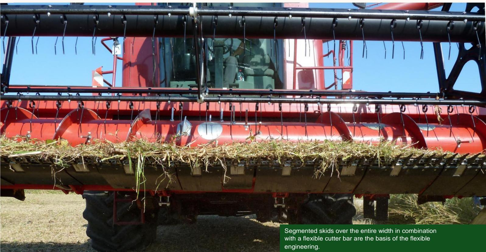
Segmented skids over the entire width in combination with a flexible cutter bar are the basis of the flexible engineering.
