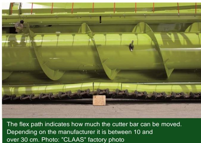
The flex path indicates how much the cutter bar can be moved. Depending on the manufacturer it is between 10 and over 30 cm. Photo: "CLAAS" factory photo
