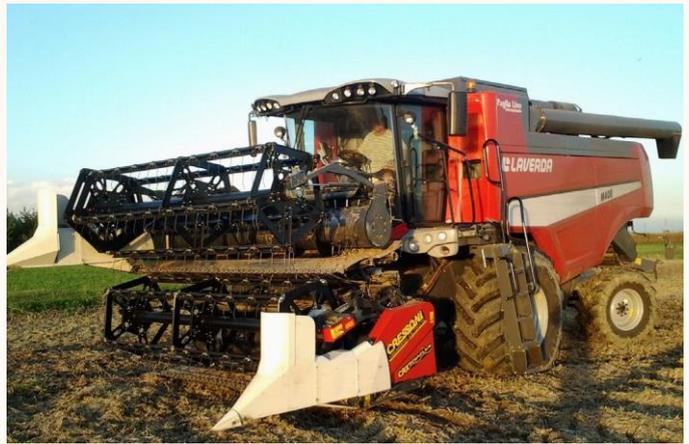
Italy is the leader in European soybean cultivation - and Cressoni has been manufacturing flex-cutting systems since the 1980s. Today, in addition to a standard machine, a special feature is a flex cutter that can be folded for transport, in working widths of up to 7.2 meters. The manufacturer advertises with an adapted intake auger, which is equipped with fingers over its entire width, enabling a better crop flow.
