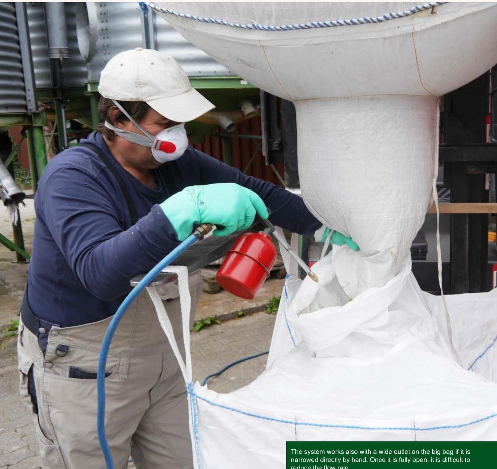
The system works also with a wide outlet on the big bag if it is narrowed directly by hand. Once it is fully open, it is difficult to reduce the flow rate.
