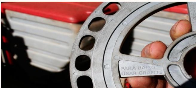
Perforated disc with the note "Use graphite": In Brazil, seed technology manufacturers sometimes specify the use of graphite in order to minimise wear of the (plastic) components in the singulation system.
