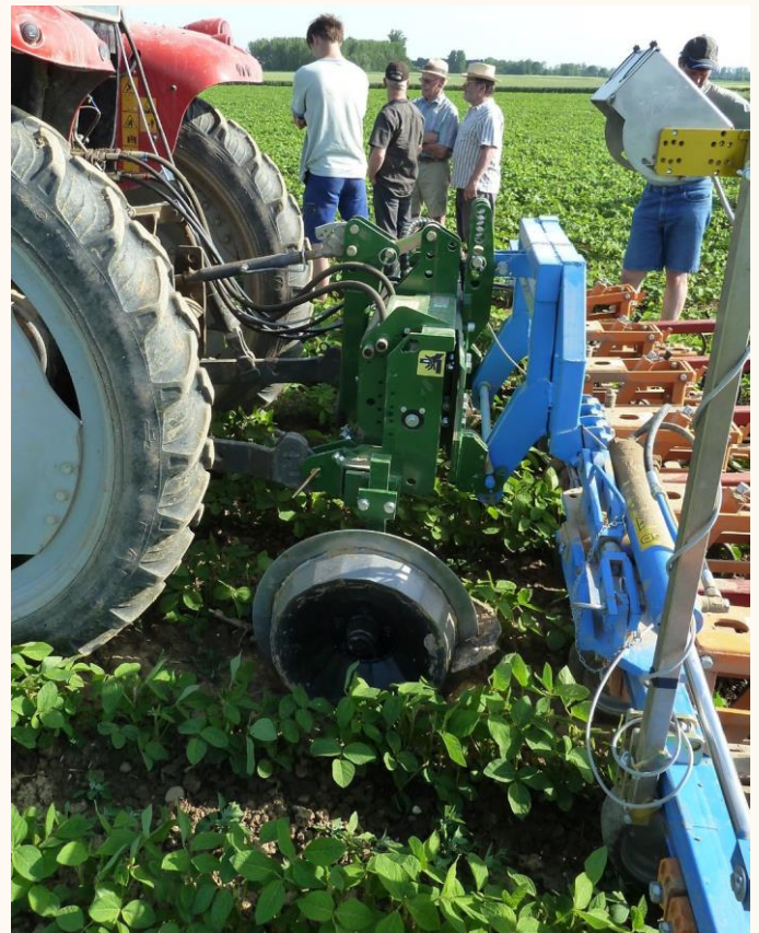
Garford side-shift control with track wheels. The tripod with the camera is mounted on the right side of the chopping frame.
